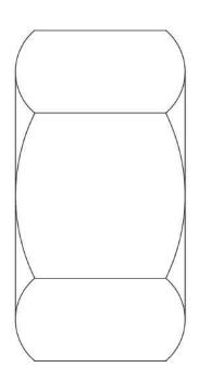
The CN-5 Standard Coil Nut is manufactured from hex stock and is available in 1/2" through 1-1/2" diameters. Dimensions are displayed in the table below. Available supplied in plain finish and electroplated galvanized.
