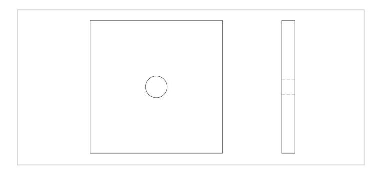
The CW-4 Flat Washers are manufactured from high carbon flat steel plate and are designed to provide the required bearing against the form members. Flat Washers are available in many sizes in both standard and heavy versions. Refer to the table below for dimensions.
