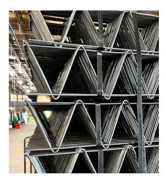
Welded Wire Girders are a trusted, cost-effective tie for integrally insulated concrete "sandwich panels" cast with a middle layer of rigid insulation between by two outer layers of concrete.
