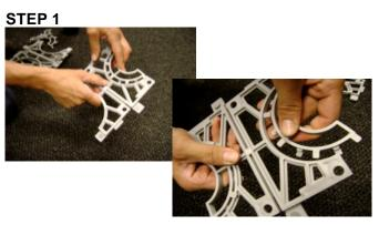
SNAP IN THE B230 BRACKET TO A B400 OR B456 BRACKET. CENTER THE TABS AND PRESS UNTIL YOU HEAR IT CLICK. REPEAT FOR THE OTHER SIDE.
