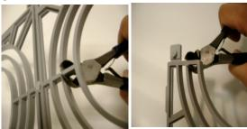
CUT SECOND RING IN FROM CENTER FOR 5" TERMINATORS AND THIRD RING FOR 6" TERMINATORS. CUT ALL THREE SECTIONS.
