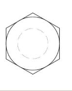
The CB-2 Coil Bolts are available in 1/2" through 1-1/2" diameters for use with Coil Ties, Coil Inserts and other Meadow Burke products furnished with coil threads. Coil Bolts are manufactured with the fast-threading, self-cleaning coil thread and are available in lengths as needed.
