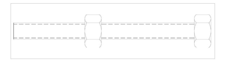
The CB-4 Adjustable Coil Bolt consists of a length of Coil Rod with a Coil Nut welded on one end and a free running Coil Nut on the threaded section. This unit simplifies ordering on projects where unusual forming conditions require numerous bolt lengths. The Adjustable Coil Bolt is available in 1/2" and 3/4" diameters in standard 18" and 24" lengths. Other diameters and lengths are available on special order.
