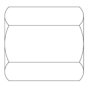
The CN-25 Heavy Coil Nutsare manufactured from hex stock like the Standard Coil Nut but is of sufficient length to develop the safe working loads required for medium and heavy form tying systems. Available supplied in plain finish and electroplated galvanized.
