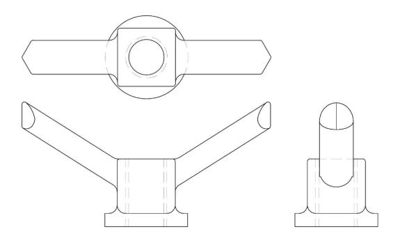
The CN-29 Coil Wing Nuts are furnished with coil thread and are available in 1/2" through 1-1/2" diameters. The ductile iron Coil Wing Nut offers high strength, speedy tightening and release.
