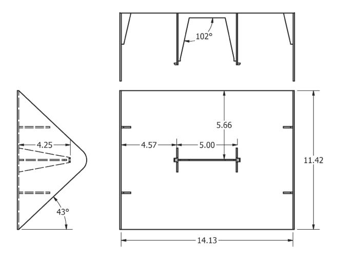
The Plastic Cover for the 30 kip Rapid-Lok is produced from a high strength, polypropylene, injection molded plastic. It has been thoroughly tested to ensure that it will perform exceptionally well, even in extreme conditions. The Plastic Cover holds its shape and resists impact damage at temperatures approaching zero and exceeding 125°F. Although it normally remains in place once installed, the Rapid-Lok Cover can be detached and reattached dozens of times if needed without deforming.
