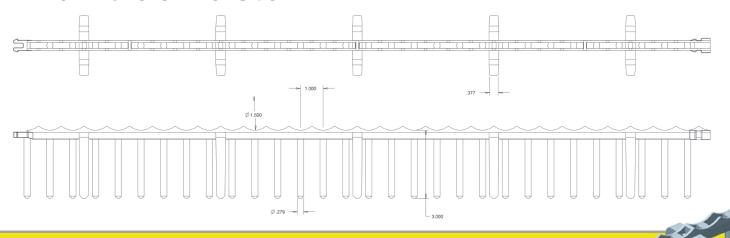
Meadow Burke X Tuff SB Slab Bolsters are the industry-leading alternative to metal rebar supports.
