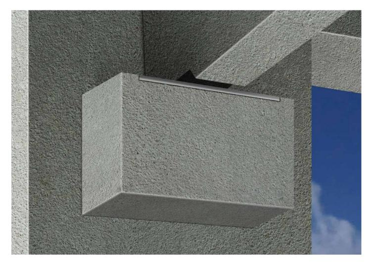
Concrete Replicated Bearing Corbel is functionally identical to the Bearing Angle but has additional studs to form a frame, allowing the casting of concrete around the corbel. The underside angle is then encased in concrete to create a traditional concrete corbel finish.
