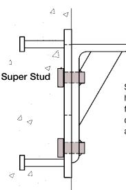
Super studs attached to the Bearing Angle have been "cold tested," configured and sized for optimum performance in all weather conditions, ensuring the load bearing capacities are met.
