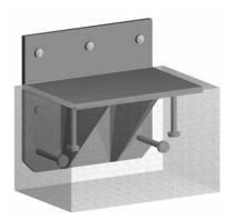
Concrete Replicated Bearing Corbel is functionally identical to the Bearing Angle but has additional studs to form a frame, allowing the casting of concrete around the corbel. The underside angle is then encased in concrete to create a traditional concrete corbel finish.
