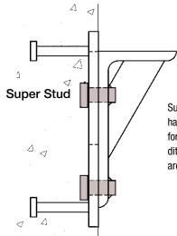
Super studs attached to the Bearing Angle have been "cold tested," configured and sized for optimum performance in all weather conditions, ensuring the load bearing capacities are met.
