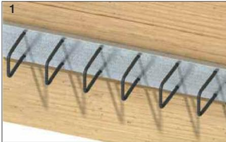
Attach the Keyway Box by nailing through the casing to the formwork or securely tie the projecting reinforcing bars to existing reinforcement. The Box should be firmly secured and tight against the formwork to avoid displacement during concrete placement.
