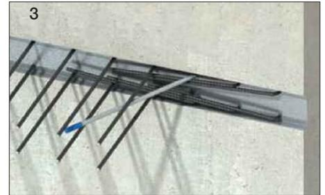
Straighten the bars using a hickey bar (cheater bar) that is slightly larger than the rebar being straightened. The bars should be straightened only once according to the procedure highlighted below. Care should be taken to avoid damage to adjacent concrete. See 'Rebar Straightening' below for additional information.
