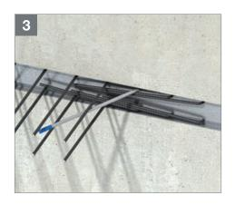
Attach the Keyway Box by nailing through the casing to the formwork or securely tie the projecting reinforcing bars to existing reinforcement. The Box should be firmly secured and tight against the formwork to avoid displacement during concrete placement.
