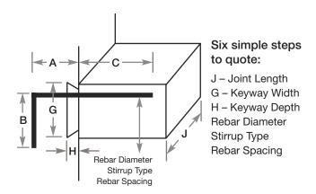
The Joint Length provides an estimate of the number of boxes needed for this application. It will also provide a guide for the length of the box itself.
