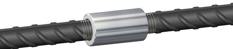
Meadow Burke BT Couplers are versatile and robust Type 1 & Type 2HS Splicing Systems used to mechanically connect rebar sections in segmental pours as an alternative to traditional dowel bars. The three-part system consists of a Splice Bar, Coupler and Setting Bar that meets the mechanical splice strength requirements of ACI-318-19 when used to splice grade 60 rebar.
